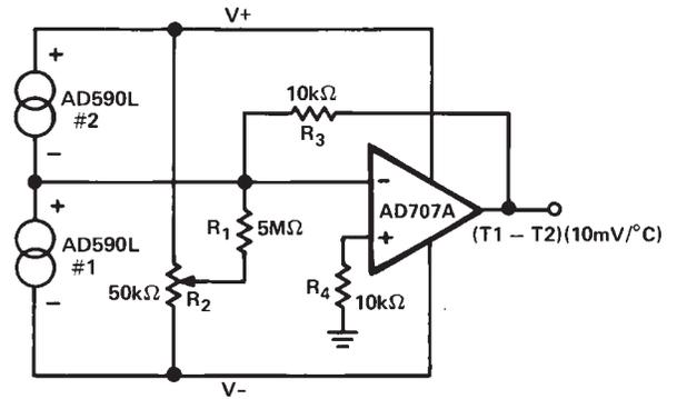
Figure 12. Differential Measurements
