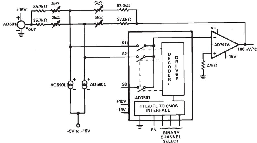
Figure 19. 8-Channel Multiplexer
