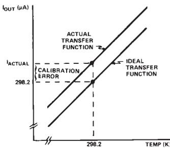
Figure 3. Calibration Error vs. Temperature
