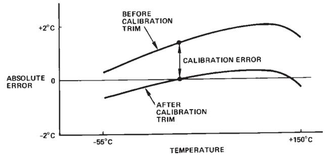
Figure 5. Effect to Scale Factor Trim on Accuracy
