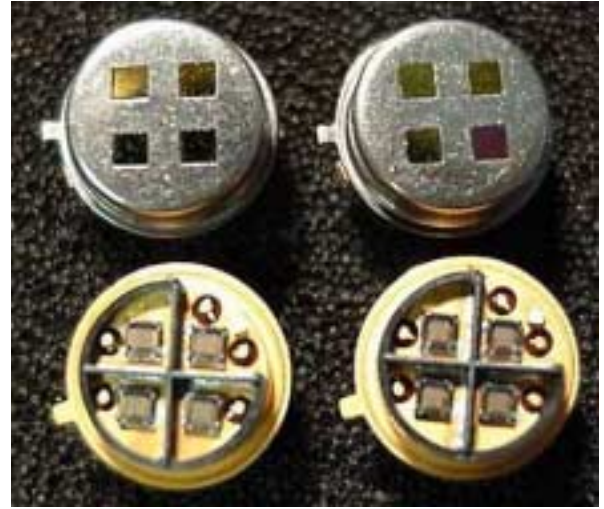
Figure 5: The quad thermopile sensor TPS 4339 houses four thermopile chips in a single TO 5 case. The open detectors in the lower row show clearly the internal aperture, that suppresses successfully any crosstalk between the four channels. Even this sensor type employs a thermistor (the small cube in the upper right position) to provide an internal temperature reference. The upper row shows closed sensors carrying four different IR bandpass gas filters.
