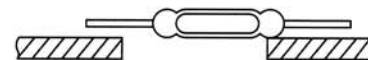
Fig. 7 Precautions to be taken when mounting reed switch on printed wiring board
