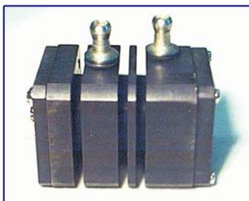
*Fig. 3.4. DX6106.C2 gas sampling cell*
