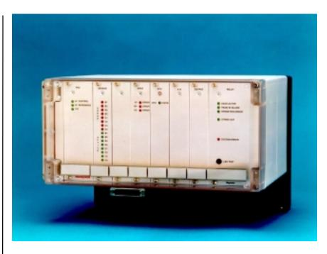
A road crossing system comprises a microprocessor based control unit and Honeywell railwheel sensors to monitor trains entering and leaving the crossing. The control unit outputs a signal to confirm that a train has cleared the crossing. This signal can then be used to start the sequence of actions to open the crossing to road traffic.
