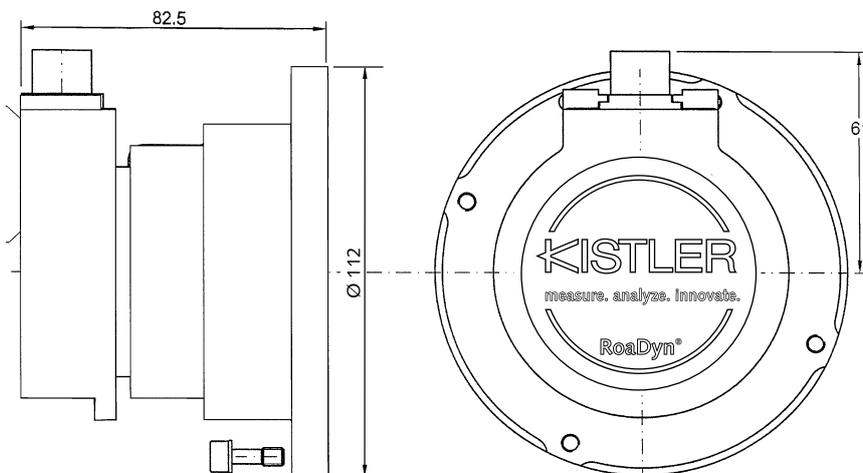
Fig. 2: Slip ring module PremiumLine Type 9873
