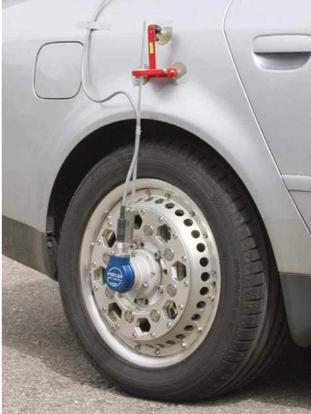
Fig. 1: Wheel torque transducer RoaDyn® P106 with slip ring module PremiumLine Type 9873
