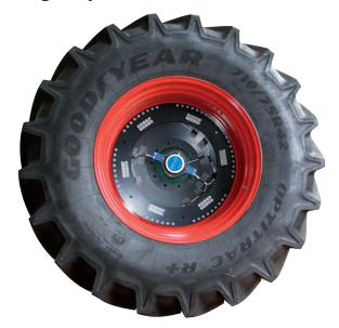
cell stores all important component parameters and prevents a misidentification of the load cell data. When the measuring system is powered up, the data of the components currently in use is imported into the connected System 2000 on-board electronics.
