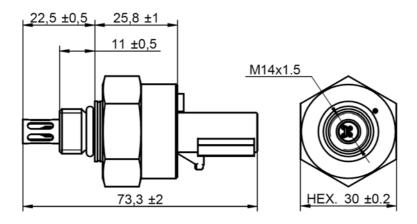
All dimensions are millimeters (mm). Mating connector type is FCI female receptacle ref. 54200409 (black-sealed). Sensor body is stainless steel.
