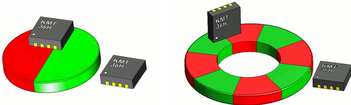
As an unique feature, the KMT36H is able to measure full 360° by utilizing an additional magnetic field which is generated by a planar coil which is located on the chip. The 180°/360° determination is done by a simple sign distinction and may be proceeded periodically or only once at power up.
