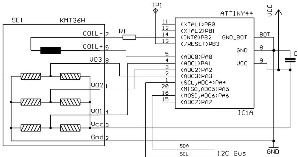
Figure 5: One exemplary hardware configuration using an Atmel ATTiny  $\mu$ C
