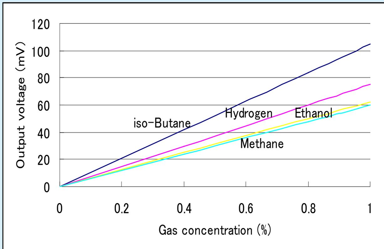
For other flammable gases, Nemoto can advise on the anticipated sensitivity of the sensor alone, but since the relative sensitivities to various gases is also dependent on the mounting arrangement within an instrument, it is always recommended that the instrument maker determines the response of the sensor to the target gas by experiment using the final product design wherever possible.
