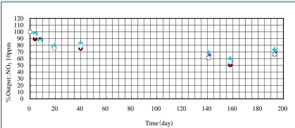
Fig. 7 : Durability in high temperature (50 degree C) with dry circumstance.
