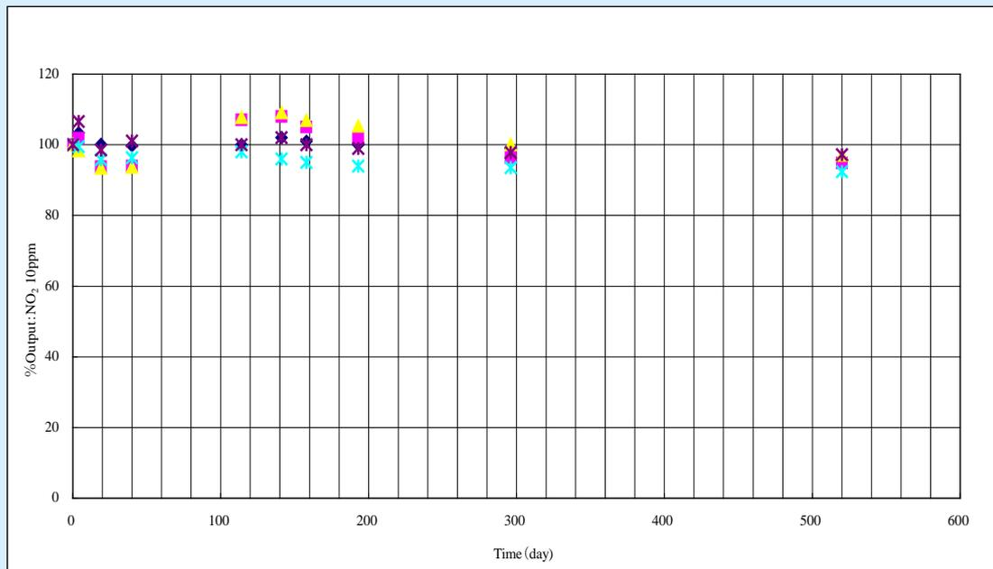
Fig.5 : Long term stability of NE4-NO2 in normal circumstance
