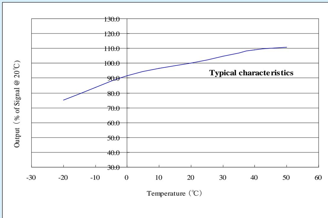
Fig. 3 : Typical temperature coefficient of NE4-NO2 (100 at 20 degree C)
