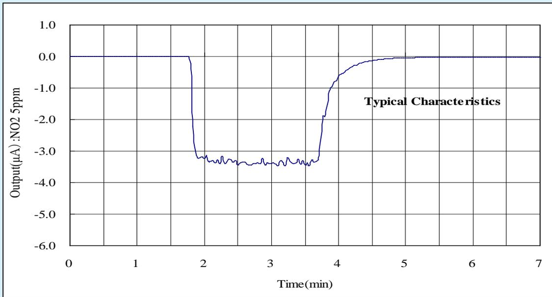
Fig.4 : Response and recovery characteristics of NE4-NO2
