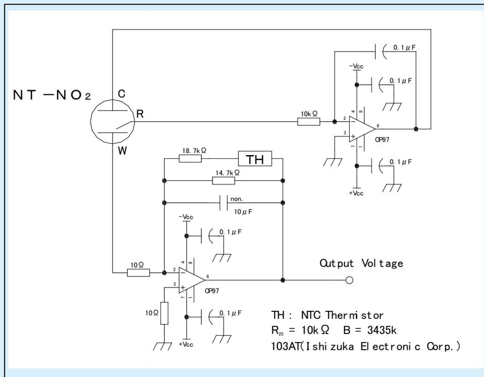
Fig. 9 : Measuring circuit diagram for evaluation
