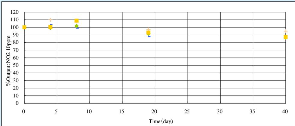
Fig. 6 : Durability in high temperature (50 degree C) and high humidity (90% RH).
