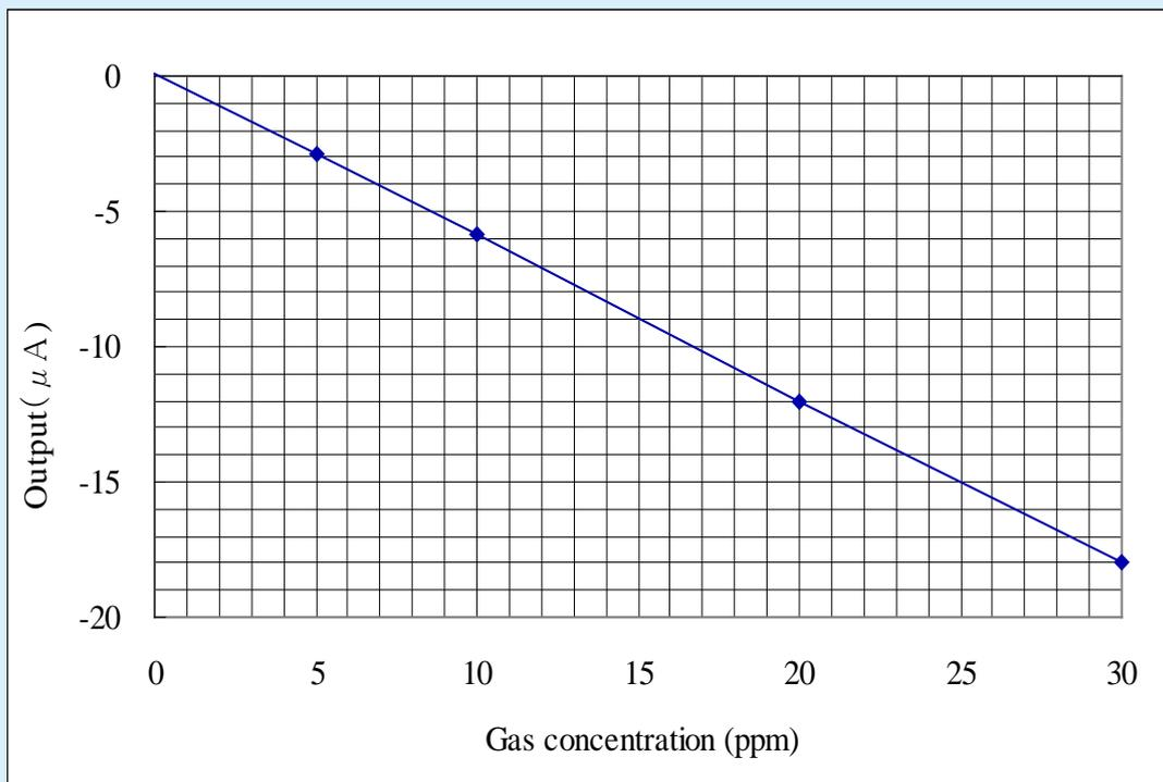
Fig.2 : Gas Sensitivity of NE4-NO2
