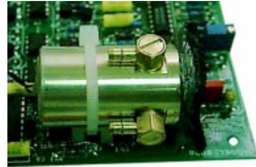
Adjustable 90° hose barb option on gas cell for lower profile
