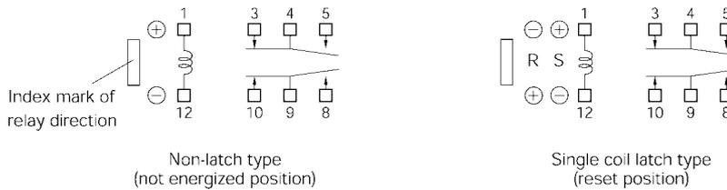
S : Coil polarity of set (operate)
