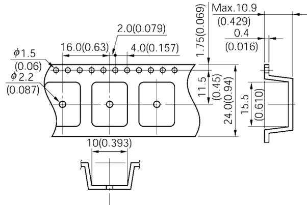
**Relay orientation mark and tape carrying direction.**
