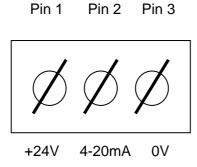
Fig. 2: Connection of AQ-Transmit. Pin 2 optionally 0-10 V.
