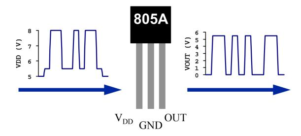
Internal temperature and offset compensation circuitry enables operation over a wide temperature range with minimal changes in accuracy and offset stability. The circuitry also rejects shifts due to mechanical stress and long-term drifts.
