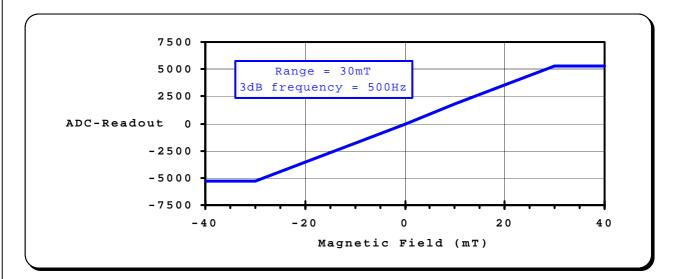
I.3 Adjustment of the Output Characteristic
