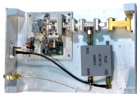
Inside view of E-band front-end of Radiometer for Castor Tokamak
