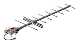
Yagi antennas are used primarily for Point-to-Point links, have a gain from 10 to 20 dBi and a horizontal beamwidth of 10 to 20 degrees.
