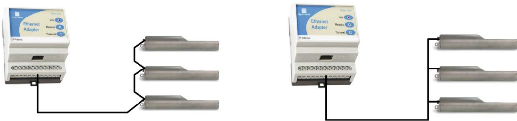
Figure 22: Correct RS485 cable networks
