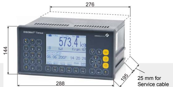
Panel-mount VEG 20450 terminal Protection class: front IP54, otherwise IP 20 Plastic 138.5 x 282 mm panel cut-out Weight: 3.5 kg
