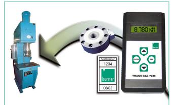
The model TRANS CAL 7280 together with a load cell is a universal reference measuring chain for the calibration of power presses. During calibration on-site the reference force is brought into the flux of the press-fit measurement system. For traceability reasons a DKD/ DAkkS- or manufacturer calibration certificate can be supplied.
