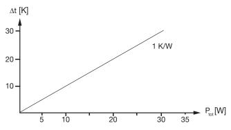
Cooling body temperature = ambient temperature + excessive temperature.
